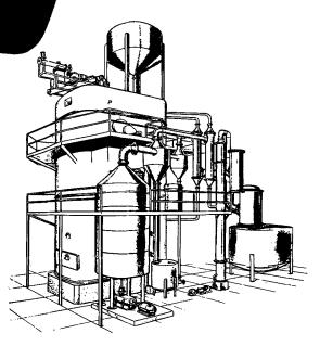
Shown above is a typical French vertical extraction plant layout. Other universal basket type extractors are available in horizontal and rectangular designs for capacities from 25 tons to 1200 tons per day.
